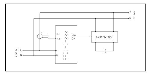
Typical single-phase power factor correction PFC1 system. Only one capacitor bank is shown for clarity. The bank switch can either be a set of solid state switches or a relay contactor. A single-phase model can also be used in a three-phase system with neutral by connecting to the detected current line and the neutral.
