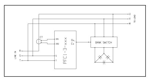
Typical three-phase power factor correction PFC1 system. Only one capacitor bank is shown for clarity. The bank switch can either be a set of solid state switches or a relay contactor. Industrial Electronics, Control, Robotics and Automation
