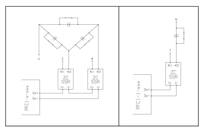
Typical solid state relay bank switch connection in three-phase (left) and single-phase (right) line systems. The SSRs must be of the zero-crossing (or line synchronized) type to ensure that the capacitors are switched in when the line voltage equals the capacitor voltage thus eliminating capacitor inrush current and extending capacitor service life. The capacitor discharging resistors are for safety only and can be any suitable value giving minimum heat dissipation while connected to the line.
