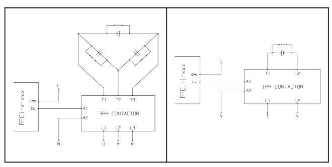
Typical contactor bank switch connection in three-phase (left) and single-phase (right) systems. The control voltage live (typically 230 VAC) is switched to activate the contactor coil.
